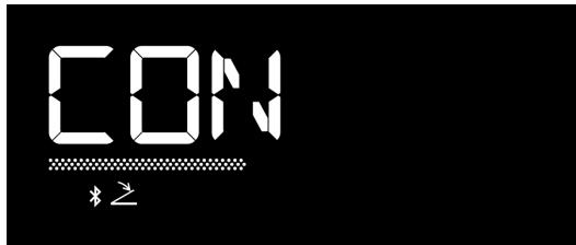
"CONNECT" is displayed,  $\ast \geq$  flashes, and the progress bar is displayed repeatedly. The foot control is automatically connected to the control unit.
