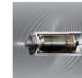
The micromotor in the VOLVERE i7 handpiece has no core and generates less rotary momentum. This contributes to the controllability of the rotation speed and reduces uneven rotation. In addition, this motor has higher power efficiency compared to a conventional motor and can maintain constant speed even at high speeds.
